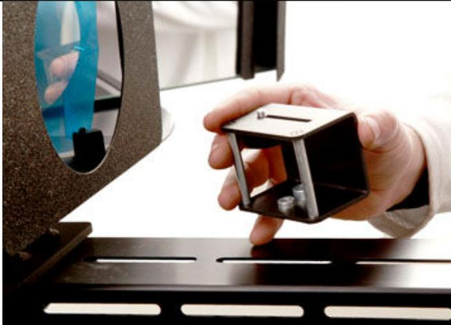
Attach RISER with either a 3/8x16 tie down screw, (recommended and included) or with a 1/4x20 tie down.
