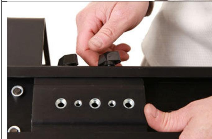
Once the initial adjustment has been made, use the knobs on the side of the 'traveling base' to secure the TRAVELER to the base plate SLED.
