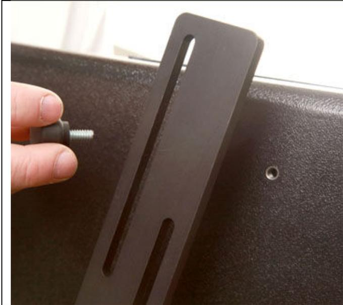
The slots in the L BRACKET allow for 4.5 inches of adjustment.
