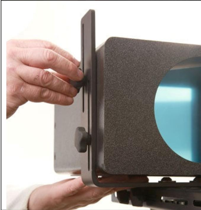
The lowest adjustment puts the optical center at 2 1/2 inches from the base plate.
